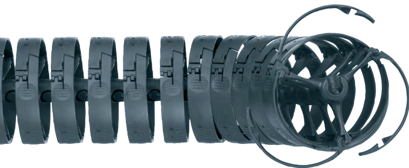
An example of a multi-axis energy chain is the triflex® R from igus®, which was specifically developed for robotics to achieve modularity, durability, safety and ease of installation: the TRCF series shown here has a special snap lock for even faster opening Source: igus® GmbH
